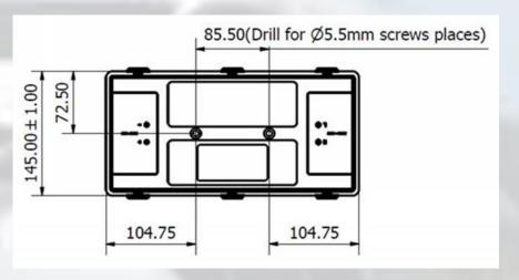
Reserve fixture clearance/space per drawing illustrated Drill two mounting (screw) holes at dia. 5.5mm
